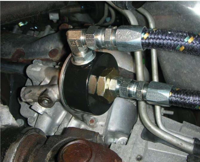
*Tighter view and different angle of adapter on engine filter mount.*
