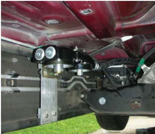
*General view of filter mount area with filter base mounted and plumbed.*
